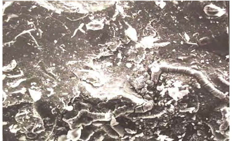
Surface profile showing contaminants and shattered Abrasive Particles impregnated into the metal profile at this magnification level
