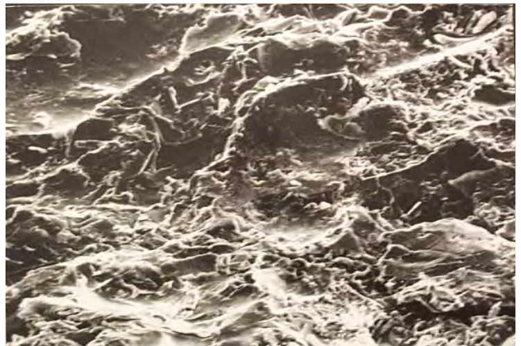
Surface profile showing no contaminants even at this magnification level
